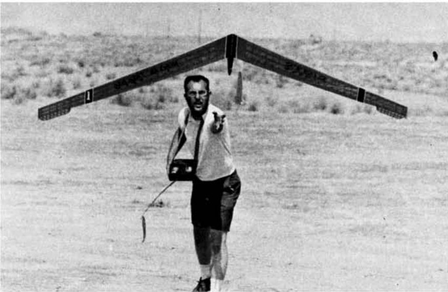
Swish and it's gone! The rubber shock cord hauls it up upward, not much pull is needed. Right: Buried piano wire reinforces the wing spar. A homesick angel in the glide.
