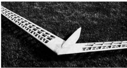
Question not the backward body, it balances. A hand-hold for launching. At left and below: the delicate framework, spars tapering toward tips.
